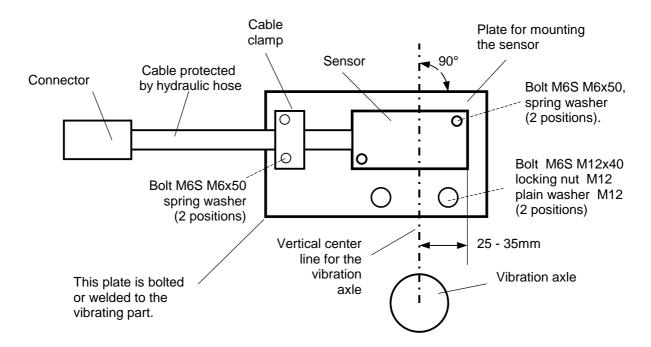
The sensor is the device that converts the acceleration of the vibrating drum into an electrical signal. The electrical signal is used by the processor to determine the CMV(Compaction Meter Value), which is a relative value for the degree of compaction.
