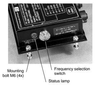
The processor is the part in the compaction meter system that determines the CMV(Compaction Meter Value) from the drum sensor signal.
