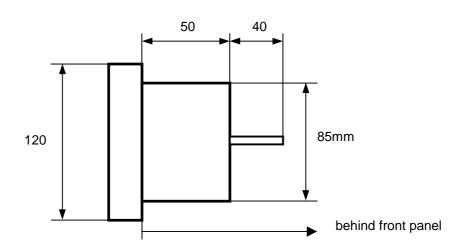
For mounting the instrument a hole with diameter 87mm has to be cut in the front panel.
